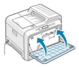
8 Using the handle, completely open the left cover until it is at right angles to the main frame and the toner cartridges are ejected.
